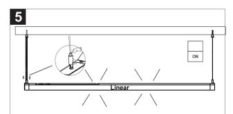
5.Press the Pedestal to adjust the height of rope, Change the CCT and watts Via external dip-switch (See B.Function), and then finish the installation.
