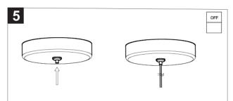
5. Press the steel wire rope holder as shown in the figure, and then insert the stainless steel wire into the inner hole of the steel wire rope holder; The mounting height of the lamp could be adjusted by this steel wire rope holder.
