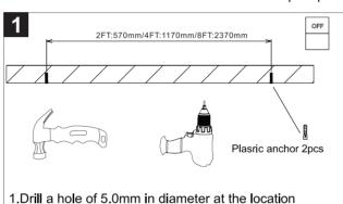
required for installation. Then install the plastic anchor
