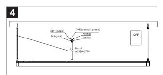
4. Turn off the wall switch, connect L,N,GND,DIM+ and DIM- of AC input wire to L,N,GND,DIM+ and DIM-respectively of AC terminal.
