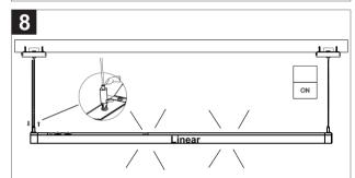
8. Press the Pedestal to adjust the height of rope, Change the CCT and watts Via external dip-switch (See B. Function), and then finish the installation.
