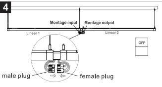
②Connect the male plug of Linear 1 and female plug of Linear 2, insert the linkable bracket to the Linear 2 make them seamless linkable together.
