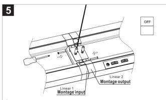
⑤ Check the status after linked make sure no any gap between two linears, and fix with screws.
