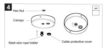
4. Insert the steel wire rope holder into the middle hole of the canopy and tighten the steel wire rope holder with hex nut; Clip the cable protective cover into the AC line hole of the canopy.
