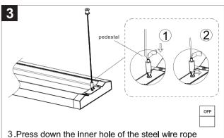
3. Press down the inner hole of the steel wire rope pedestal, let the steel wire rope go through the hole.
