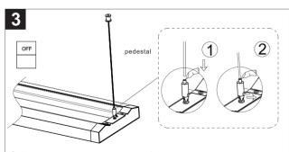
3 .Press down the inner hole of the steel wire rope pedestal, let the steel wire rope go through the hole.
