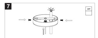
7. Adjust the length of the AC input cable, align the side hole of the canopy and the M mounting bracket as shown in the figure, then tighten the screw.
