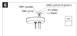
Insert the AC input cable through the cable protective cover and connect it with the AC line by the corresponding connection wire with L, N, GND.
